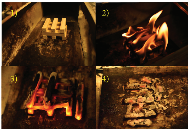
Figure 2. Evolution of a typical burn where 1) is the pre-burn period, 2) is the flaming combustion period, 3) is the smoldering period and, 4) is near the end of the experiment.
